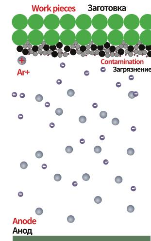
Ar+ plasma bombardment on work pieces to remove contamination layer
